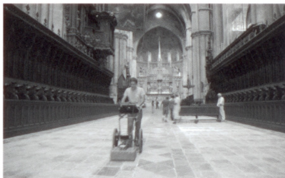
Fig. 7 - Picture showing the record of a GPR profile along the central nave of the cathedral.
