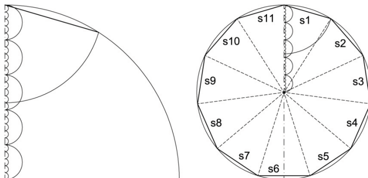
Fig. 6: Simple approximation to a hendecagon construction.
