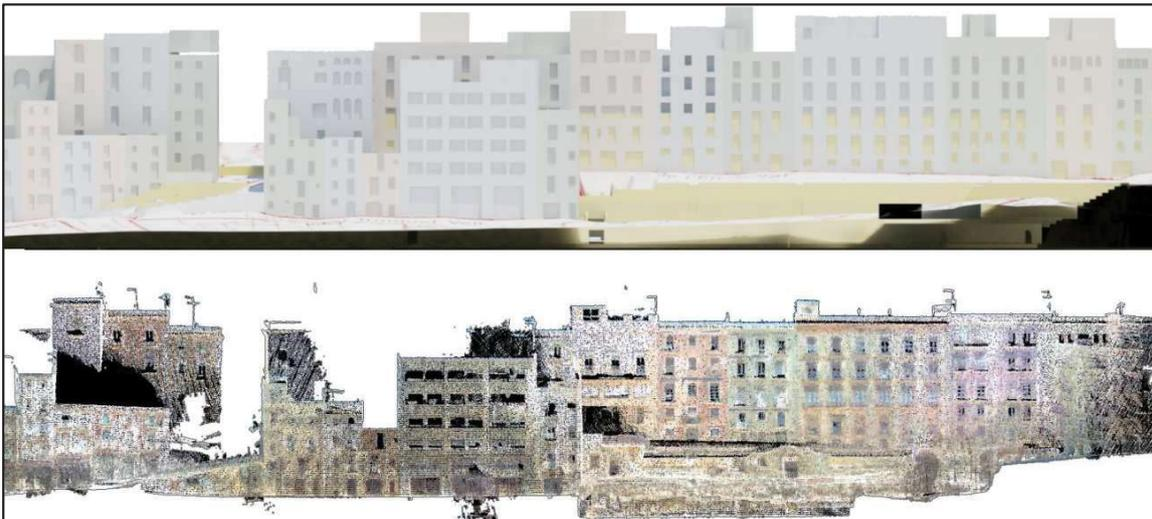
Figure 3. Scanning of *Trinquet Vell* street and three-dimensional reconstruction.
